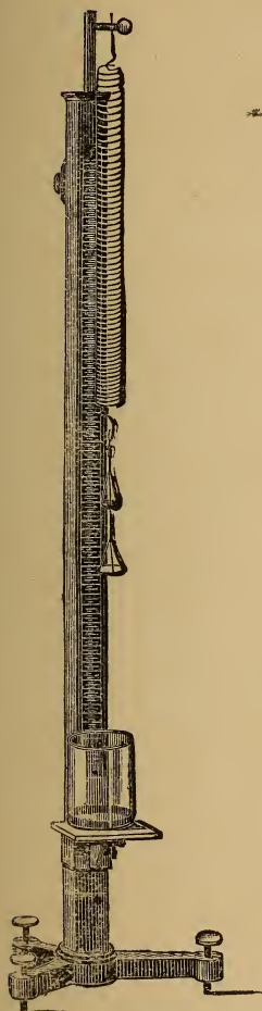
Fig. 82. PROF. JOLLY'S APPARATUS FOR DETERMINING THE SPECIFIC GRAVITY OF MINERALS.
